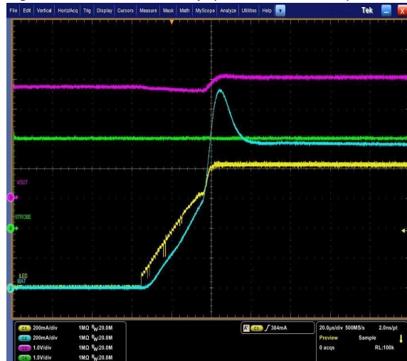
Figure 9. I_{VIN} , ILED Startup ( I_{LED\_OUT}=800mA )
