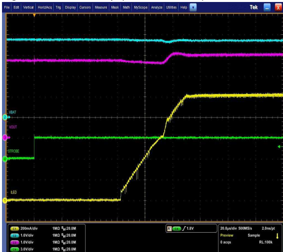
Figure 8. ILED Startup ( I_{LED\_OUT}=1.0A )
