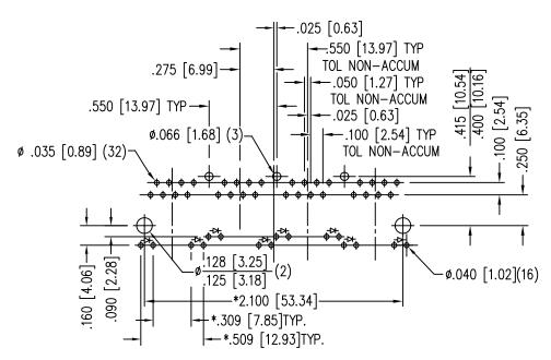
P.C.B. RECOMMENDED HOLE LAYOUT SEEN FROM COMPONENT SIDE TOLERANCE ±.003 [0.08] UNLESS OTHERWISE SPECIFIED
