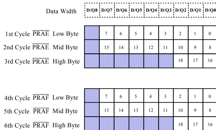
FQV2113, FQV2103, FQV293 Parallel Offset Write/Read Cycles for x9 Bus Width Condition Applies to: FQV293 x9 to x9 mode or FQV2113, FQV2103 for all modes
