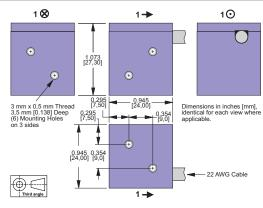
6061-T6 aluminum case with electroless nickel finish plus integrated cable with shield bonded at the case
