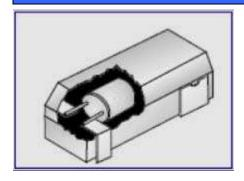
The FPXLF layout is one of the earliest conversions from Thru-Hole, to surface mount. As such, the 2 terminations on the right are not used for anything in the circuit. The pads are there only to provide additional mechanical adherence to the circuit board.
