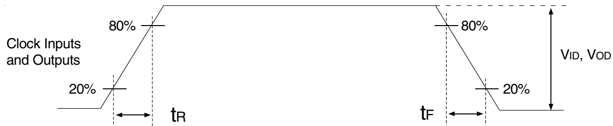
Figure 8. Input and Output Slew Rates
