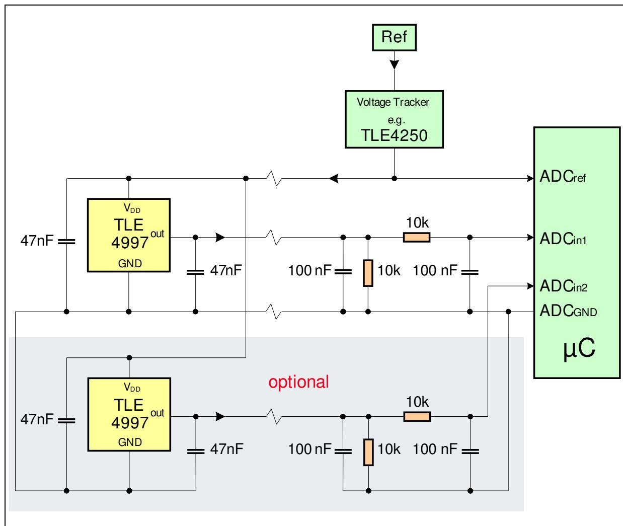
**Figure 10 Application Circuit**
