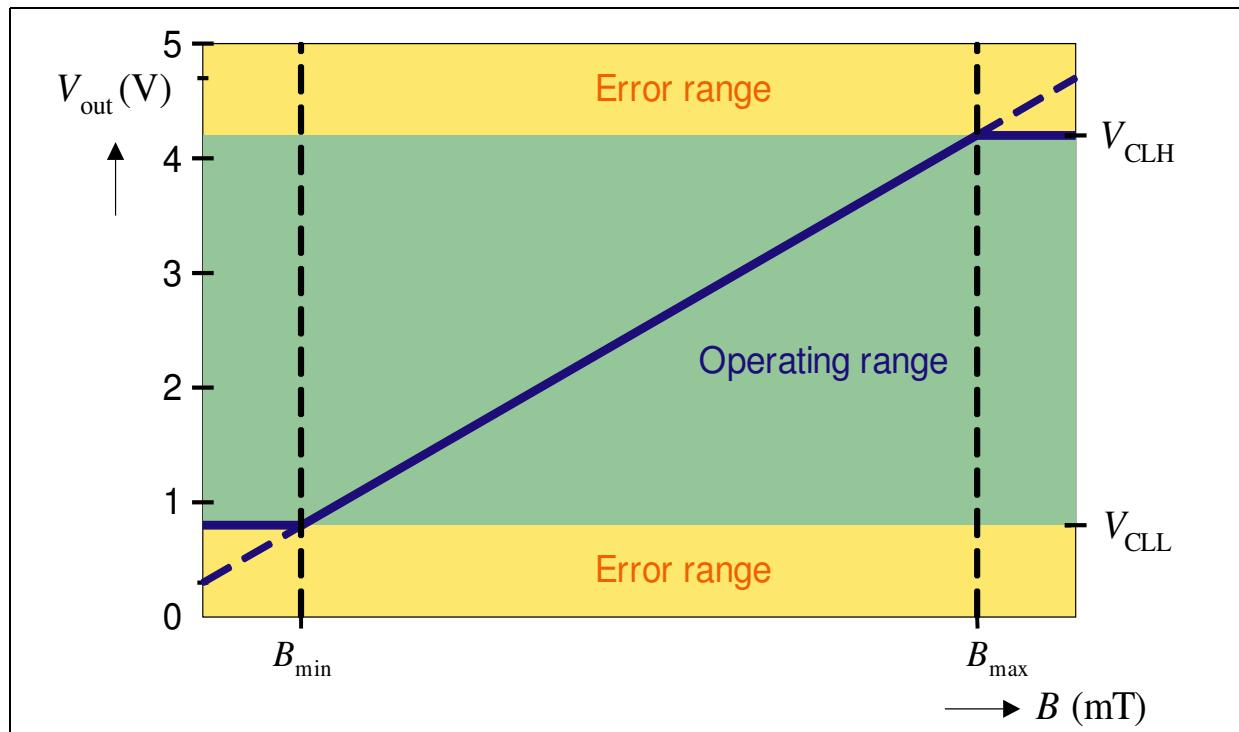
**Figure 8 Clamping Example**
