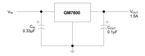
For a positive regulator, a 0.33µF bypass capacitor should be used on the input terminals. While not necessary for stability, an output capacitor of 0.1µF may be used to improve the transient response of the regulator. These capacitors should be on or as near as possible to the regulator terminals .
