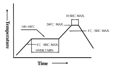
3. DIP soldering (Wave Soldering):
