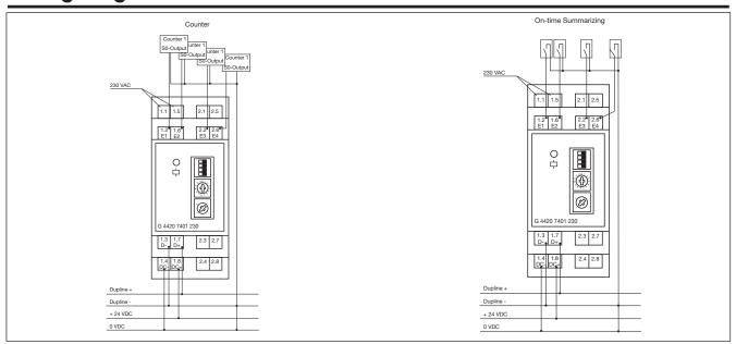
In order to avoid disturbances, the length of the cable between the counter inputs of G4420 7401 and the impulse output should not exceed 5 m. NOTE: The G4420 7401 724 is pure DC-supplied. The G4420 7401 230 has the possibility of two powersupplies, both a DC and a AC. If using the DC Supply, the minus of the supply is used as common wire for the inputs of the module.
