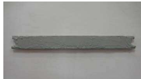
Thermal glue on rear surface
