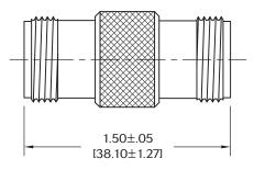
Note: Dimensions in Brackets are Expressed in Millimeters and are for Reference Only. Design specifications are subject to change without notice. Contact factory for technical specifications before purchasing or use.
