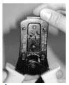
4. Press pre-positioner downward firmly for contact handles alignment. (crimp area should be facing upward).
