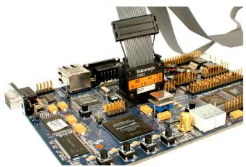
The P5934 is 34-channel mictor probe with quick connect/disconnect and a positive latching mechanism to ensure a secure, reliable connection.
