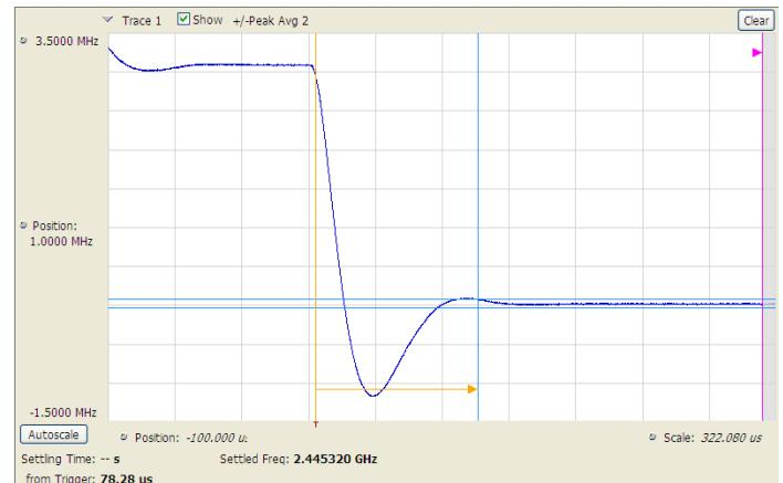
**Settling time measurements** (Opt. 12) are easy and automated. The user can select measurement bandwidth, tolerance bands, reference frequency (auto or manual), and establish up to 3 tolerance bands vs. time for Pass/Fail testing. Settling time may be referenced to external or internal trigger, and from the last settled frequency or phase. In the illustration, frequency settling time for a hopped oscillator is measured from an external trigger point from the device under test.
