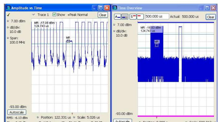
**Advanced Triggers and Swept DPX** combines the revolutionary DPX Density™ Trigger with the ability to trigger on runt pulses and apply time qualification to any trigger. The runt trigger seen here can be used to track down nonconforming pulses in a pulse train, greatly reducing time to insight. Time qualification can be used to separate ranging pulses from higher resolution pulses in a radar signal, or trigger only on signals that remain on longer than a specified time.
