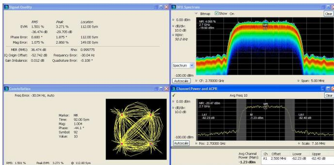
Time-correlated, multidomain views provide a new level of insight into design or operational problems not possible with conventional analysis solutions. Here, ACLR and Vector Modulation Quality (Opt. 21) are performed on a single acquisition, combined with the continuous monitoring of the DPX® spectrum display.
