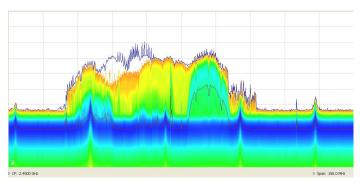
Advanced Triggers, Swept DPX, and Zero Span (Opt. 200) provides superior swept spectrum analysis for transient signals. Here, a 150 MHz swath of spectrum is swept across the ISM band. Multiple WLAN signals are seen, and narrow signals seen in the blue peak-hold trace are Bluetooth access probes. Multiple interfering signals are seen below the analyzers noise level in the multi-color DPX display.
