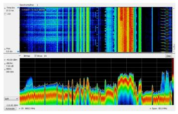
DPX Spectrograms (Opt. 200) provide gap-free spectral monitoring for up to days at a time. 60,000 traces can be recorded and reviewed, with resolution per line adjustable from 110  $\mu s$  to 6400 s.
