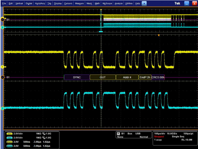
Triggering on a specific OUT Token packet on a USB full-speed serial bus. A bus waveform provides decoded packet content including Start, Sync, PID, Address, End Point, CRC, Data values, and Stop.
