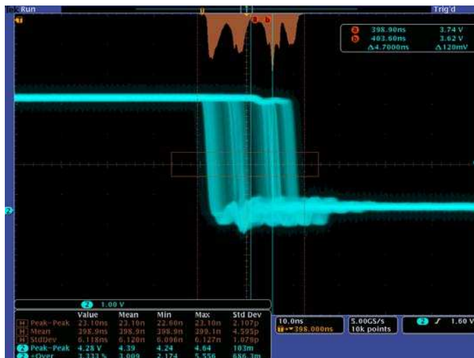
Analyze – Waveform histogram of a falling edge showing the distribution of edge position (jitter) over time. Included are numeric measurements made on the waveform histogram data. A comprehensive set of integrated analysis tools speeds verification of your design's performance.
