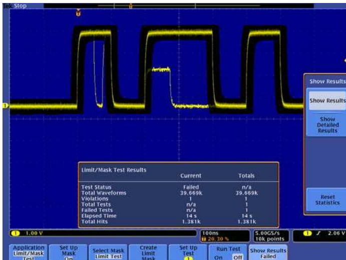
Limit Test showing a mask created from a golden waveform and compared against a live signal. Results showing statistical information about the test are displayed.
