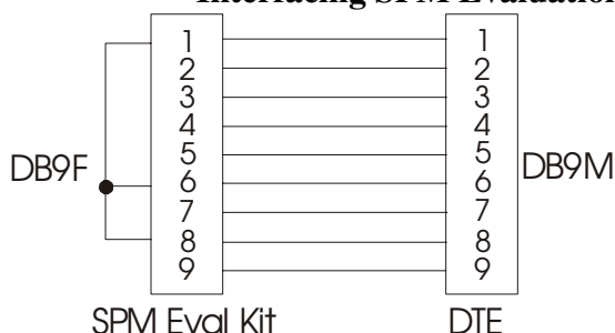
Figure 4: DB9M-DB9F straight through modem cable
