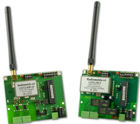
Figure 1: CTA28 application boards
