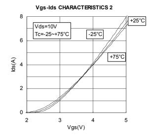
RoHS Compliance, Silicon MOSFET Power Transistor,175MHz,30W
