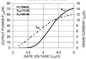
RoHS Compliance, 135-175MHz 60W 12.5V, 3 Stage Amp. For MOBILE RADIO
