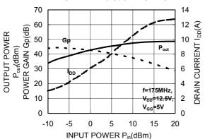
RoHS Compliance, 135-175MHz 60W 12.5V, 3 Stage Amp. For MOBILE RADIO
