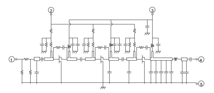
RoHS Compliance, 135-175MHz 60W 12.5V, 3 Stage Amp. For MOBILE RADIO
