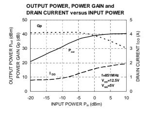
RoHS Compliance, 820-851MHz 6W 12.5V, 3 Stage Amp. For MOBILE RADIO
