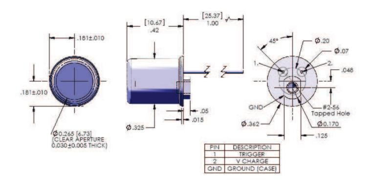
Package is subject to change depending on required internal components to achieve specified parameters. Dimensions: inches [mm]
