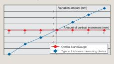
At a vertical movement of 6 mm, the Optical NanoGauge has variations below 0.1 nm, while a typical thickness measuring device exhibits variations up to 8 nm.
