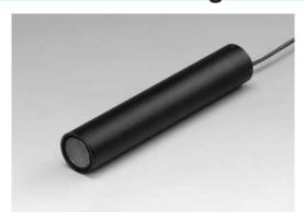
The H11123 is a photon counting head device consisting of a 28-mm (1-1/8") diameter head-on photomultiplier tube, a high-speed photon counting circuit, and a high-voltage power supply circuit. The high voltage power supply for photomultiplier tube and the discrimination level are preset to optimum values, allowing photon counting measurement by just connecting a +5 V supply. The H11123 can operate at high count rate.
