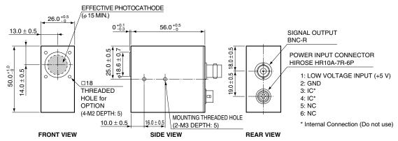
Power cable with connector (HIROSE HR10A-7P-6S) is supplied with H7828 series
