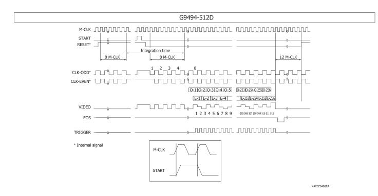
Note: When used with the G9494-256D, M-CLK equals CLK-ODD. When used with the G9494-512D, M-CLK is divided by 2, and CLK-ODD and CLK-EVEN are generated with complementary timing and output while each is shifted by half the CLK period. This means that the G9494-256D and 9494-512D operate at the same data rate when a same frequency M-CLK is input.
