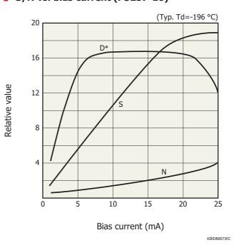
The detector must be operated in a range where the D\* becomes max.
