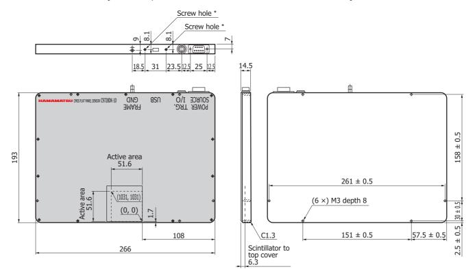
Top cover material including window is carbon fiber (1.0 mm thickness). Weight: 1.3 kg  $\,$
