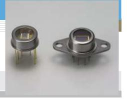
S2592/S3477 series sensors combine a UV to near infrared Si photodiode with a thermoelectric cooler. A thermistor is also included in the same package to sense the Si photodiode chip temperature. This allows stable operation over long periods of time, making these sensors suitable for low-light-level detection where a high S/N is required.
