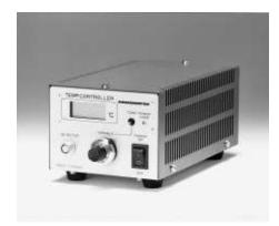
By adjusting the current flowing through the thermoelectric cooler in a onestage or two-stage thermoelectrically cooled detector, C1103-04 maintains the detector element at a constant temperature. The cooling temperature can be easily set by using the control knob on the front panel.
