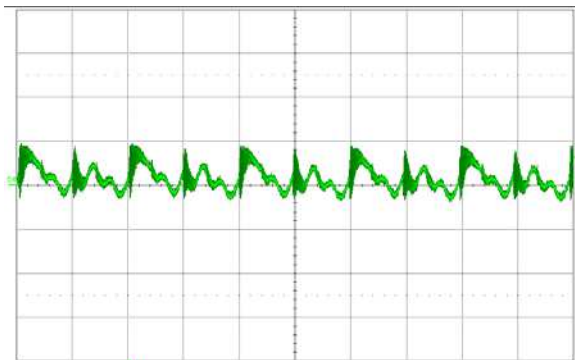
Figure 13. Output voltage ripple (20 mV/div.) at full rated load current into a resistive load with C_o = 10\mu\text{F} tantalum + 1μF ceramic and V_{in} = 48 V. Time scale: 2 μs/div.
