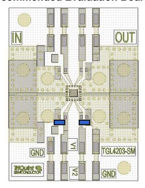
1nF(size 0402) capacitors for DC decoupling Board material is 8 mil ROGERS RO4003
