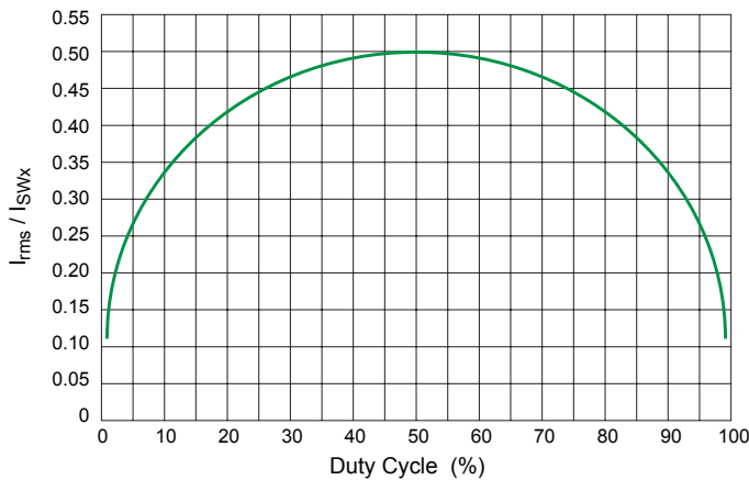
Figure 23. Input capacitor ripple versus duty cycle
