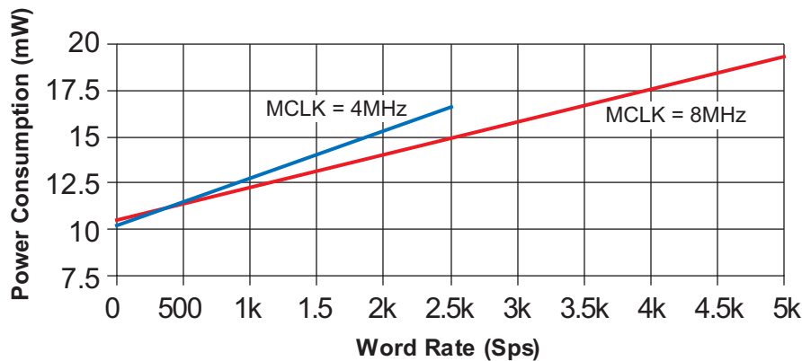
Figure 6. Power Consumption vs. Conversion Rate
