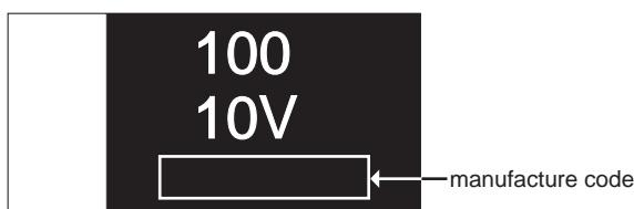
note 2) voltage code and capacitance code are variable with parts number
