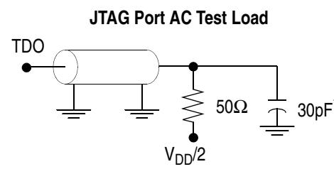
\* Distributed Test Jig Capacitance
