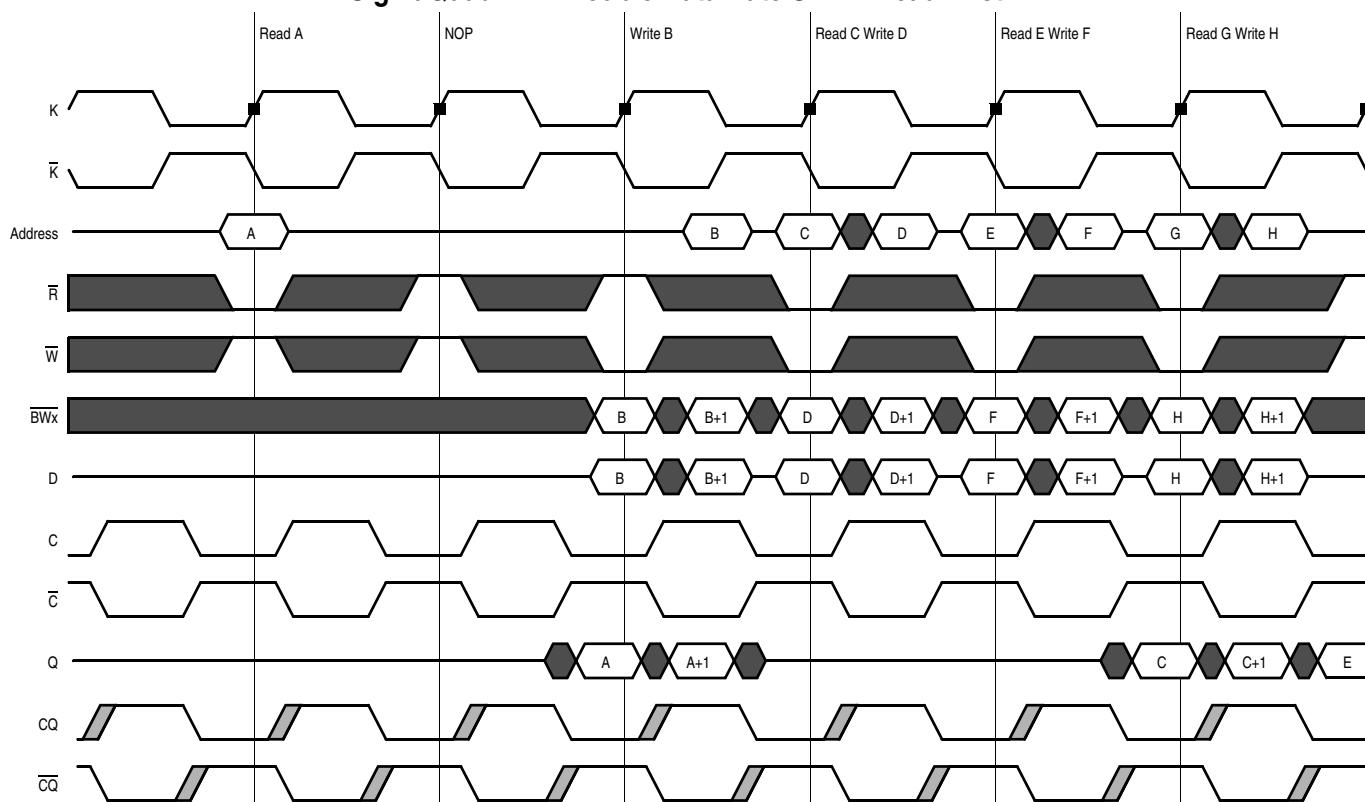
**SigmaQuad-II B2 SRAM DDR Write**
