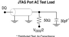
\* Distributed Test Jig Capacitance
