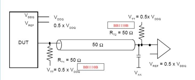
SSTL\_2, Class I, buffer with symmetrically double parallel terminated output load
