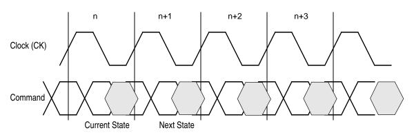
Current State and Next State Definition for: Pipelined and Flow Through Read Write Control State Diagram
