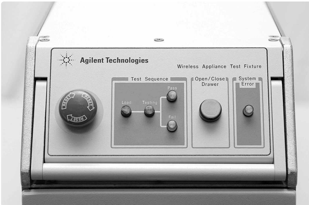
Figure 8. E8421A wireless test fixture front panel
