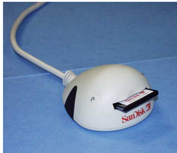
Figure 6: SanDisk® Image Mate adapter for fast data exchange of high number of OTDR trace files between E6000C Mini OTDR and N3900A Modular Network Tester.
