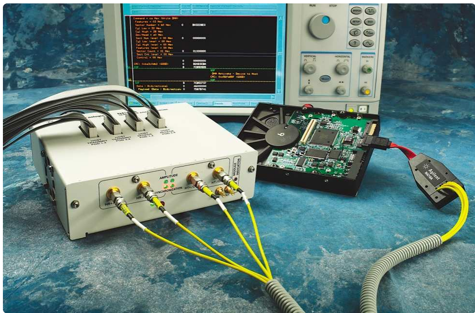
Figure 1. The N4219A packet analysis probe and the N4218A interposer provide digital design engineers who design SATA products with a complete system for debugging SATA system hardware and software
