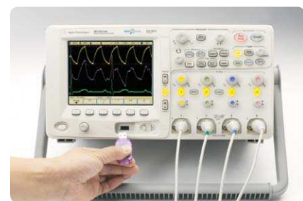
Figure 2. To permanently store data, you can save it to an external USB memory device through the oscilloscope's front panel USB port.
