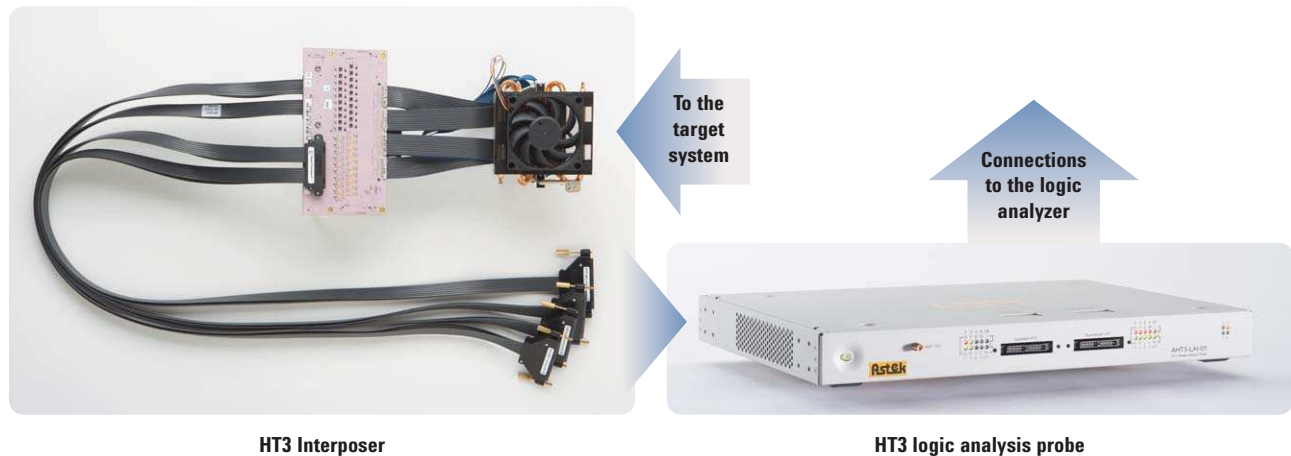
Figure 4. DC coupled interposer probe sends buffered copy of the link data from the target to the HT3 logic analysis probe.
