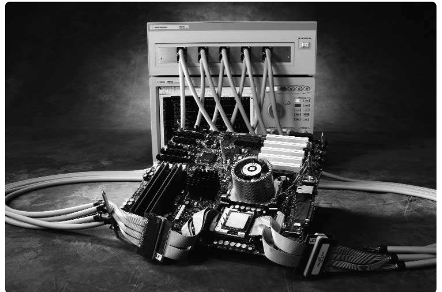
Figure 1. Intel Xeon processor analysis probe
