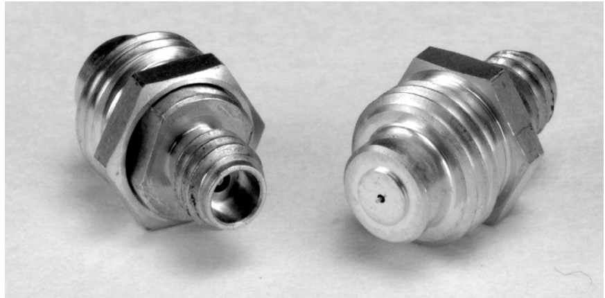
A pair of 1.0 mm female connector launch assemblies. Left: 1.0 mm female connector end Right: Package end with 0.162 mm diameter pin
