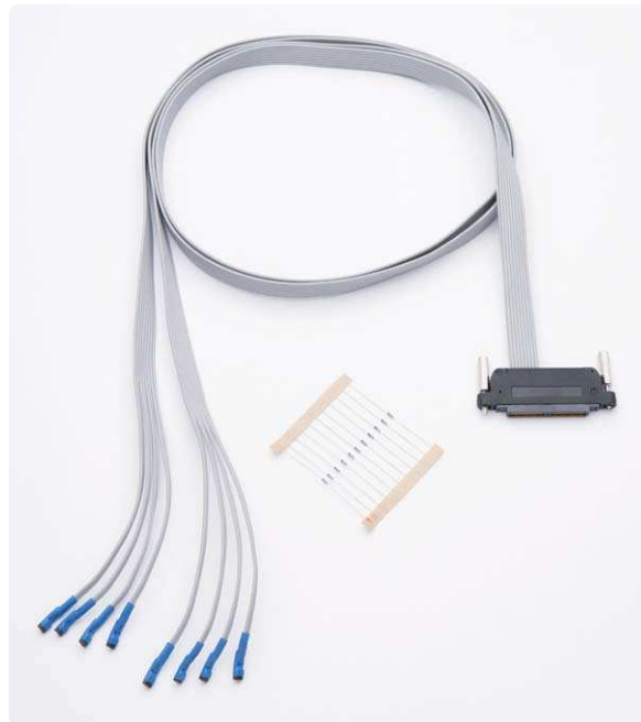
Figure 3. A flying lead set lets you probe signals individually.
