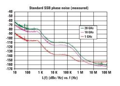
Standard phase noise performance with I/Q modulation on I
