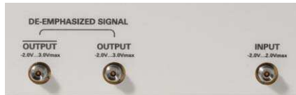
Figure 6: Front panel connectors of N4916A
